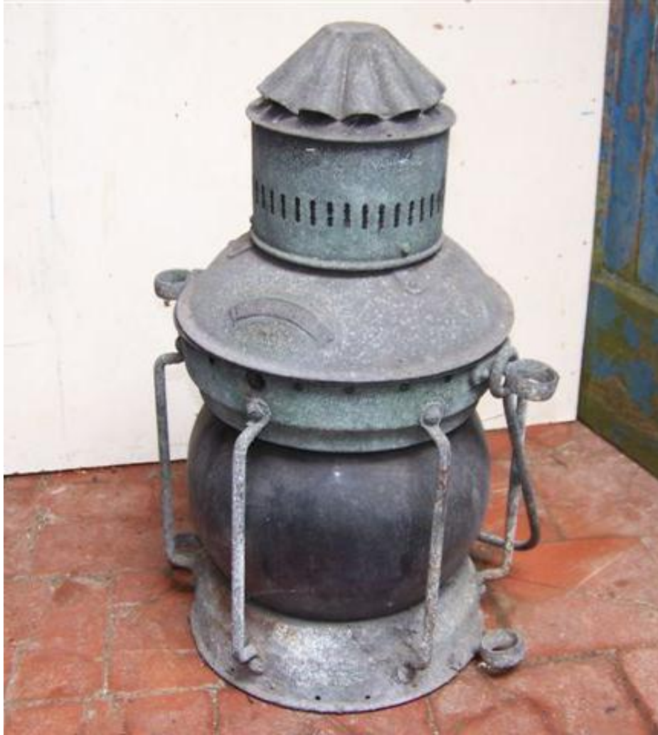
A paraffin-fuelled anchor light, used on the dumb barges until the 1960s
