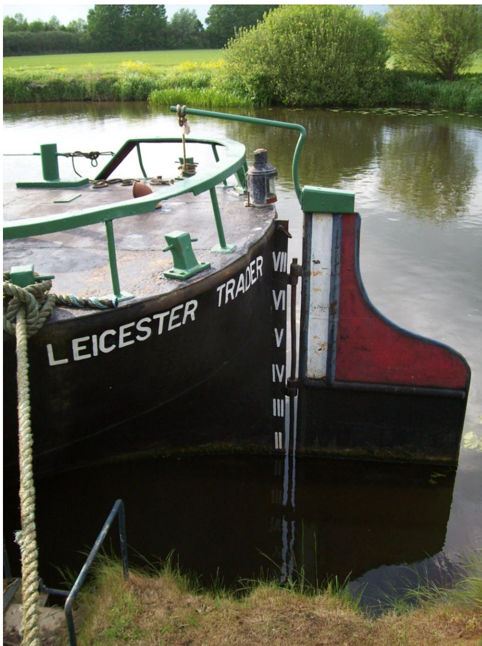
Leicester Trader's stern, showing the rudder and draught marks
